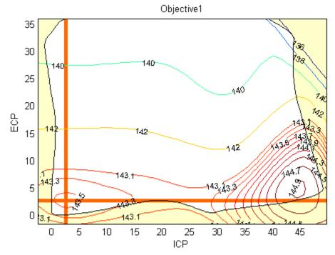
To inspect contour plots for many pairs of free variables, you can configure the optimization output view to display multiple contour plots simultaneously. Simultaneous display can help locate those runs that have converged to a local optimum.
