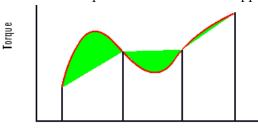
The green shaded areas show the error between the interpolated table values and the model using the initial breakpoints.
