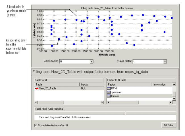
The upper pane displays the breakpoints of your table as crosses and the operating points where there is data as blue dots. Data sets display the points in the experimental data, not the values at the breakpoints. You can inspect the spread of the data compared to the breakpoints of your table before you fill the table.
