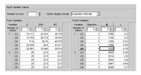
The preceding figure shows an optimization that runs twice (**Number of runs** has been set to 2, and the left column under **Number of Values** shows 2 runs). Each run contains five operating points (as shown in brackets in the right column under **Number of Values**).
