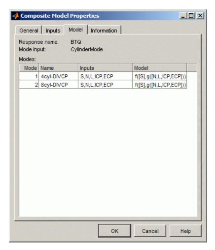
For composite models created by combining point-by-point models, use the Composite Model Properties dialog box to view which modes are available for each operating point, as shown in the next figure.
