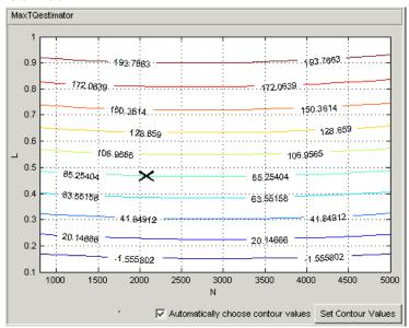
You can specify where you want contours by clicking **Set Contour Values**. Use the check box to return to automatic contour value selection. You can also control number of contours, filling and labels in the display options (toolbar or **View** menu).
