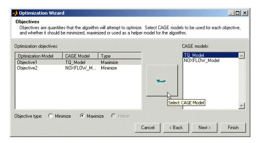
Here you can select which models from your session you want to use for the optimization, and whether you want to maximize or minimize the model output. The fopton algorithm is for single objectives, so you can only maximize or minimize one model. The NBI or gamultiobj algorithms can evaluate multiple objectives. For example, you might want to maximize torque while minimizing NOX emissions. Remember you can also define constraints later, for example, using emissions requirements.
