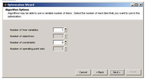
The foptcon algorithm can only have a single objective, so this control is not enabled. Choose the number of free variables and constraints you require. You can also add constraints later.
