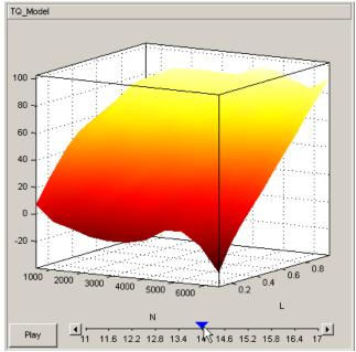
The movie option allows you to see an evaluation over two variables at successive values of a third variable. For example, a model of torque might have speed (N), load (L), and air/fuel ratio (A) as inputs.
