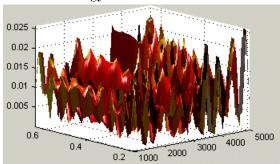
To display the error, select one of the Error options from the **Plot Type** drop-down menu. This changes the graph to display the error between the model and the strategy.
