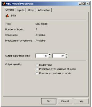
Here you can see the model type (such as MBC model or function model), the number of inputs, and the availability of constraints and Prediction Error.
