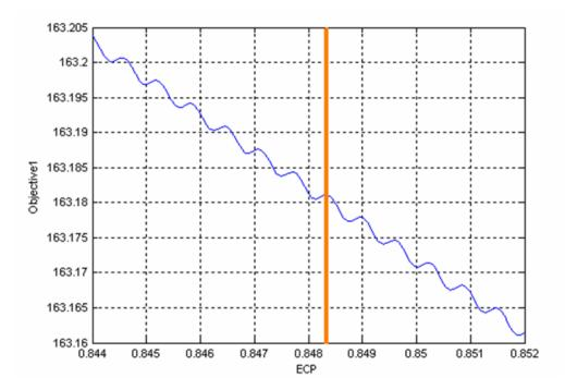
You can see that the model is noisy and the optimizer has (correctly) returned a local maximum of the model. However, this result is a maximum of the noise component in the model and not the physical component. If the noise is not behavior of the physical system, then you should remodel the noisy models in the Model Browser. The CAGE Import tool can be used to replace the noisy models with the results of the remodeling and the optimization can be rerun.
