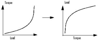
Inverting a table allows you to link a *forward strategy* to a *backward strategy*; that is, swapping inputs and outputs. This process is desirable when you have a "forward" strategy, for example predicting torque as a function of speed and load, and you want to reverse this relationship in a "backward strategy" to find out what value of load would give a particular torque at a certain speed.
