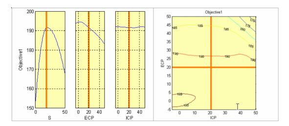
In this case, the problem appears to be over constrained because the plots are entirely shaded yellow. You can check the constraint summary table or the output table to identify if constraints are met. Also inspect the constraint summary and constraint graphs.
