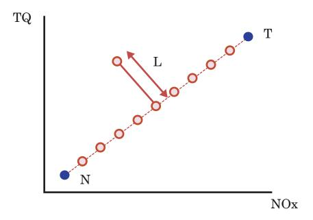
The figure above shows spacing of the points between the along the (n-1) surface. The algorithm tries to maximize the distance  $\mathbb L$  along the normal away from the surface. The following figure shows the final solution found by the NBI algorithm.
