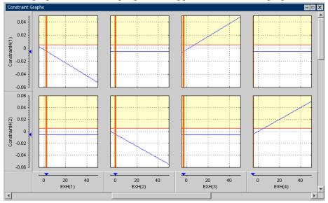
The Left Value is compared with a plot of the Right Value output on the same axes. This comparison is illustrated for the table gradient example problem. Consider the top-left graph in the figure shown. Constraint4(1) is the first Left Value  $(rg_I^{inc})$  of the table gradient constraint in the example problem. Recall that this can be written as
