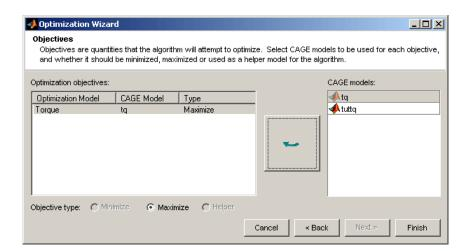
CAGE switches to the **Optimization** view and the new Optimization node appears in the tree.
