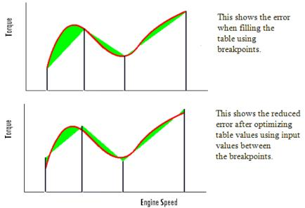
To see the difference between optimizing table values and optimizing the positions of breakpoints, compare with the illustration in "How CAGE Optimizes Normalizer Breakpoints" on page 4-5.
