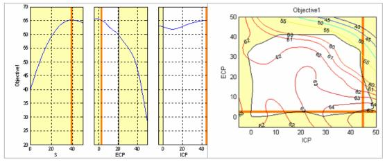
In this case, the optimizer has almost found the optimal solution for this run. If this optimizer has taken a long time to run, then as this solution is almost optimal it is probably worth marking as acceptable (select the **Accept** box in the Optimization Results table for this run).
