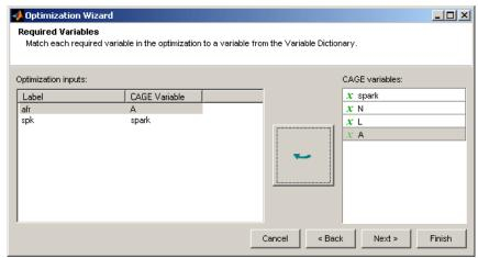
5 The next screen of the wizard automatically shows the Torque model selected and Maximize chosen; these are specified in the function. Select tq in the CAGE model list and click the button to match it with the Torque optimization model, then click Finish.
