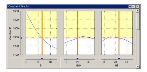
This example shows the constraint EXTEMP ≤ 1290° C.
