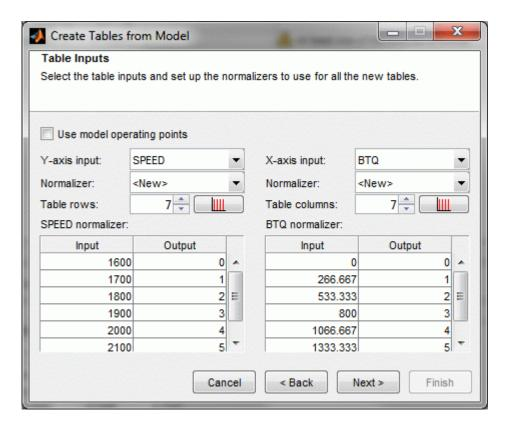
If you have selected a point-by-point model, CAGE automatically selects the check box to **Use model operating points** for the table normalizers. You can clear the check box if you want to select different normalizers.
