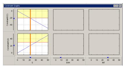
The constraint graphs for a range constraint shows how the Left Value of each output of a range constraint depends on the free variables in the optimization. The Left Value is compared with a plot of the Right Value output on the same axes. This comparison is illustrated for the example problem at the second run, as shown in the top left graph.
