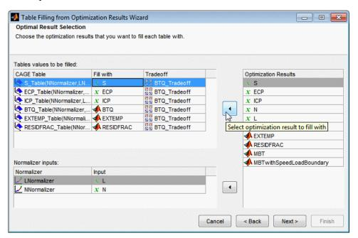
Verify the **Normalizer inputs** show the correct inputs. You might need to specify the **Normalizer inputs** to match with optimization results, if you are filling tables with different inputs to your optimization operating points. See "Table Filling When Optimization Operating Point Inputs Differ from Table Inputs" on page 7-14.
