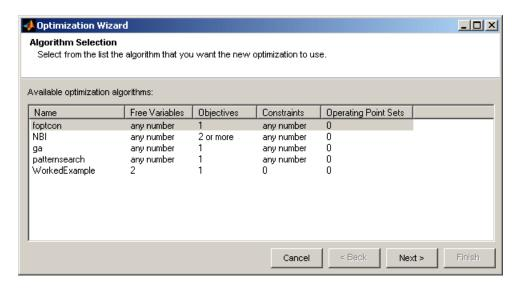
The first four algorithm choices in the list are standard routines you can use for constrained single and multiobjective optimization.
