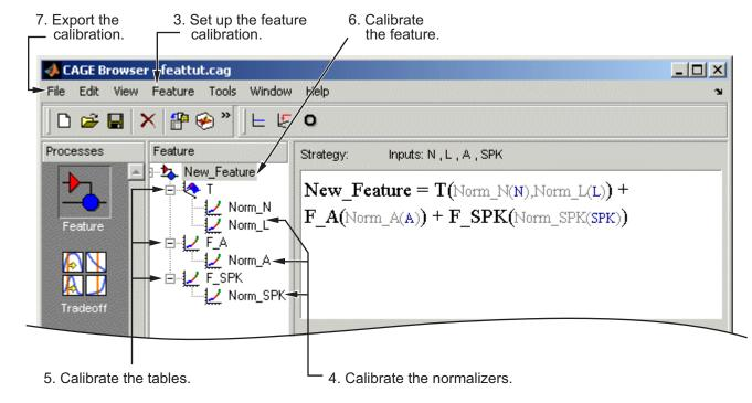
The normalizers, tables, and features form a hierarchy of nodes, each with its own view and toolbar. The feature view is shown.
