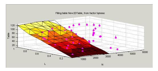
This display shows the table filled with the experimental points overlaid as purple dots.
